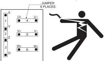
Figure 12. Voltage Change-Over Board
